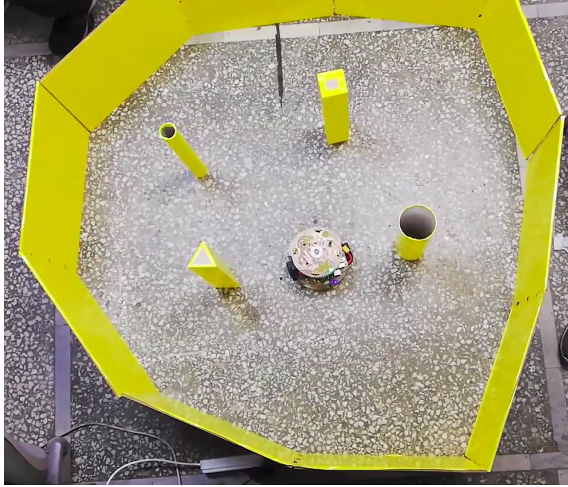
Figure 14: Real life environment to test SLAM algorithms
